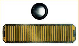
**On the left: The accordion-like pleated foil membrane** of the X-ART tweeter effectively draws air in and squeezes it out of its folds. Slight foil motions can be translated into vast air motions that way. The picture on the right shows how much larger the area of an unfolded X-ART diaphragm is compared to a 1" dome tweeter.
