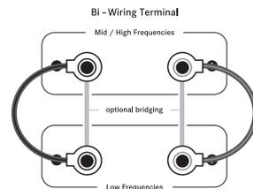
In order to bi-wire the speakers remove the bridges and connect an additional length of speaker cable to the second pair of speaker terminals. At the amplifier, terminate both red and both black conductors into the same binding post, (or separate binding posts if provided).
