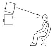
In case you need to position the speaker in a significant lower or higher position, the monitor should be angled accordingly.
