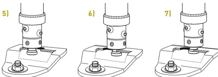
→ Loosen the tightened screw **G** (Fig. 8) and slide the retaining ring **F** downwards until it rests on the top of the mounting accessory (Fig. 9).
