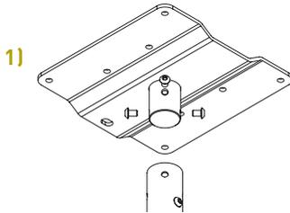
→ Place the telescopic boom **E** on the support plate cylinder **B** and secure it with 4 of the lens screws **C**. Tighten the lens screws with retaining ring **F**. The torque should be 15 Nm (see fig. 2 and 3).
