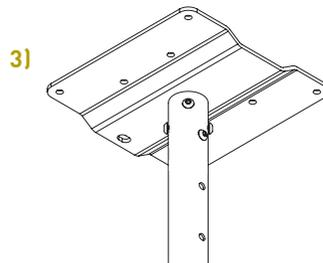
→ Adjust the height of telescopic boom **E** and secure its inner part. Only use these settings whilst no other accessory or speaker system is attached to the ceiling mount.
