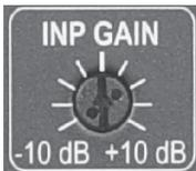
To adapt to different signal levels, the voltage that is needed to drive the unit to its maximum SPL (sound pressure level), is variable in a  $\pm 10$  dB range.
