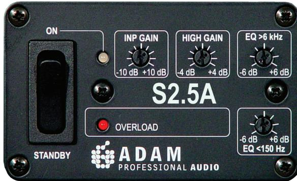
The Back Panel Controls allow the speaker to be adapted to different listening and room requirements. There are controls for:
