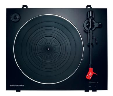
Aside from the platter, the tone arm is the most important device on a turntable to achieve an even and steady playback. The AT-LP3 offers a balanced tone arm with a solid and adjustable counterweight to get the right tension on your stylus. Although the arm itself is straight, the headshell is mounted at an angle to ensure the stylus sits comfortably in the record grooves with the least amount of side pressure from the outer regions right into the centre of the record.
