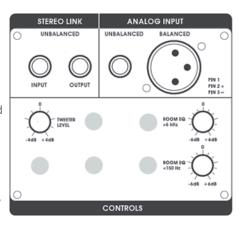
professional studios or at home. While each powered monitor has a volume adjustment knob, Adam provided a special Stereo-link feature. This allows users to adjust the volume of both loudspeakers with only one control to ensure a balanced volume level. The A5 is offered in flat black or high quality piano finishes (black and white).
