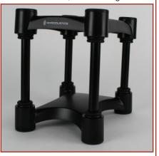
The unit is made up of six components: A lower platform that stands on four rubber feet, an upper rectangular frame that carries the speaker cabinet, and the connecting four vertical tubes, one in each corner. The user can choose a shorter 4" or taller 8" set of tubes. The isolation is provided by friction-fit rubberized sleeves in the corners of the platform and the upper frame where the tubes fit snugly but with minimal transmission of vibrations.
