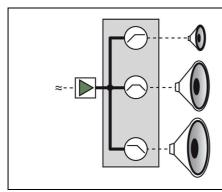
Figure 2: Schematic representation of the signal's run in a passive three way loudspeaker
