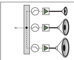
Figure 4: Schematic representation of the signal's run in an active three way loudspeaker
