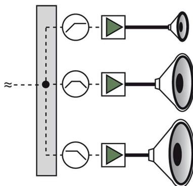
*Figure 4: Schematic representation of the signal's run in an active three way loudspeaker*
