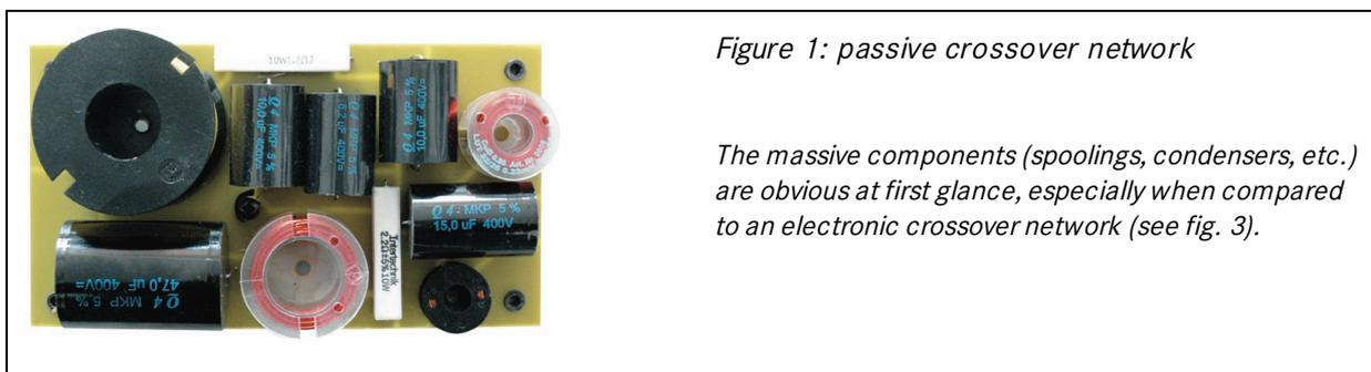
Having been divided into these different bands, the electrical signals are being sent to the corresponding drivers, which transform them into mechanical vibration, i.e.: sound waves.
